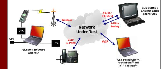
Providing clear, uninterrupted voice is critical in Network and Echo Cancellation development. GL's Voice Quality Testing (VQT), accessed through an easy to use GUI interface, provides the voice quality measurement and analysis tools for all types of networks carrying voice traffic. Typical network applications include VoIP systems, PSTN, ATM networks, Frame Relay, and Wireless Networks.
