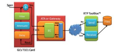
Figure: EC Testing ATAs & Gateways with T1/E1 Interface
