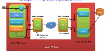
Figure: Automated EC Testing of Gateways
