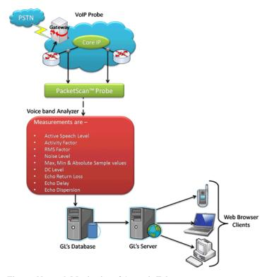
Figure: Network Monitoring of Acoustic Echo
