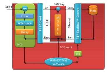
Figure: EC Testing of ATAs & Gateways - VoIP & TDM interfaces
